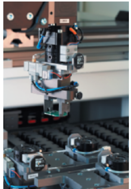
Simple and light-weight grippers for PCB handling are cost-saving and guarantee shortest cycle time with highest flexibility.
