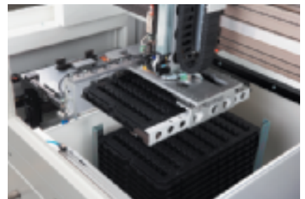
The linear motor based tray handling system detects the status of the tray with a light barrier and guarantees trouble-free operation also with various types of trays.
