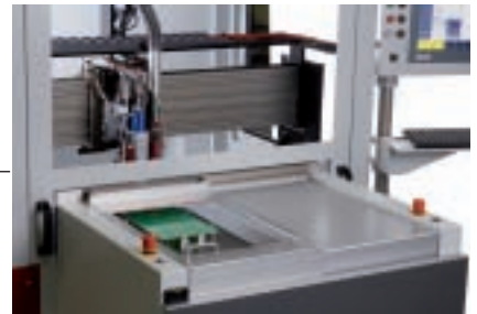
A linear motor shuttle system feeds in multi panels and removes the separated components and trimming waste.
