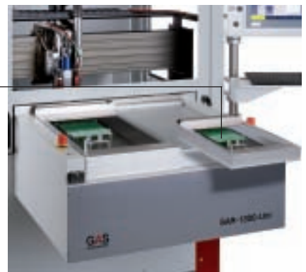
The machine can be equipped with one or two shuttle systems for panel infeed and passing back separated components and trimming waste. Customized worktables can be affixed to the shuttle mounting plate quickly and accurately. The second shuttle system can be retrofitted at any time. When equipped with a dual shuttle system, the machine offers maximum output by avoiding time lags.
