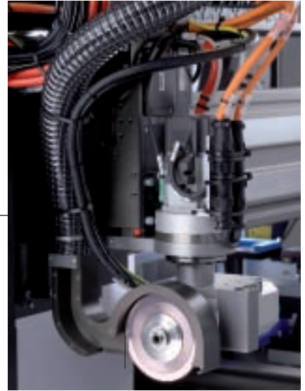
With the milling disc module, long straight crosscuts can be executed in optimum cycle times.
