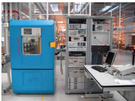
Optical test with thermal stress
