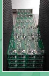
The basis of the ENGMATEC test handler is a robust knee lever system, which can be fitted both with a servo drive or with pneumatic cylinders. With the servo drive, connections can be made up to 4080 test points simultaneously on a maximum effective area of 400 x 400 mm. The contacting unit works single-sided or double-sided, also step by step for panel testing depending on requirements.
