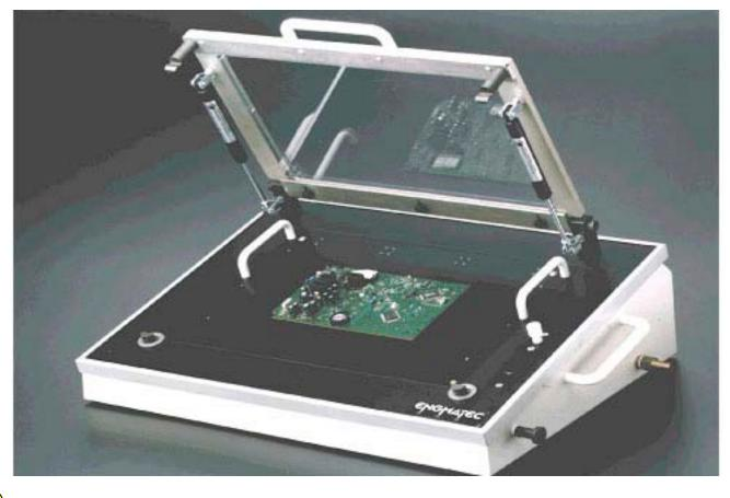
Mechanical or pneumatic adapter system with interchangeable contact pin or test item carrier plate.
