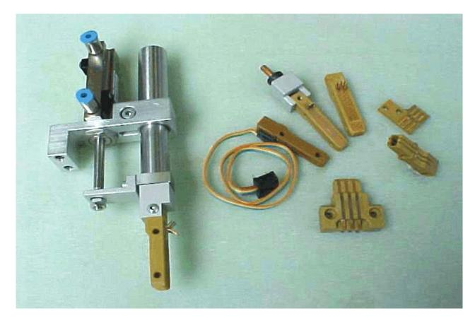
Western-Min-Plugs for contacting in 4 pin (RJ-10), 6 pin (RJ-12), 8 pin (RJ-45) and 10 pin (RJ-48) sockets
