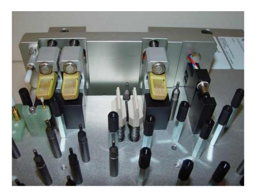
Mounted in debugging fixture:USB-Plug type A
