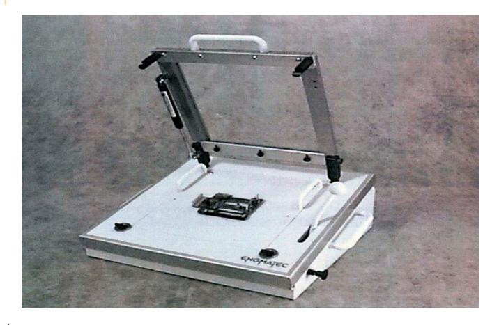
Mechanical or pneumatic adapter system with interchangeable contact pin or test item carrier plate.
