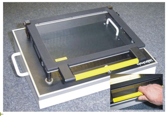
The lifting mechanism is actuated by a switch integrated into the handle.
