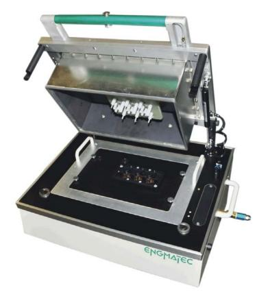
The lifting mechanism is actuated by a switch integrated into the handle.
